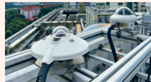
Solar irradiance sensors used in the solar forecasting model developed by SERIS. (Photo: SERIS)
