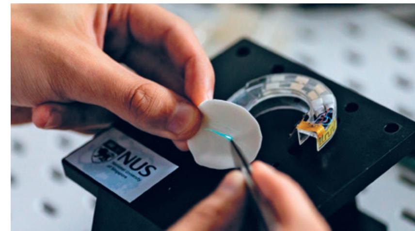
This novel bite-controlled optoelectronic system developed by NUS researchers is capable of translating complex bite patterns into data inputs with 98 per cent accuracy.
