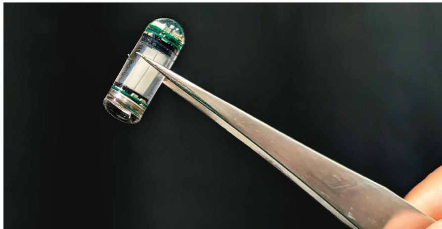
The components of the dosimeter fit into an 18mm by 7mm capsule, a common size for many supplements and medicines.
