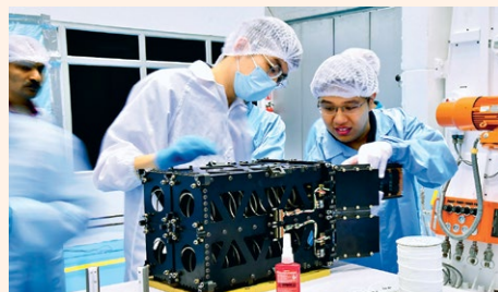
Galassia-2 project leaders Mr Eugene Ee (right) and Mr Ng Zhen Ning (Engineering '15) (left) overseeing integration of the satellite with the deployer system prior to launch.
