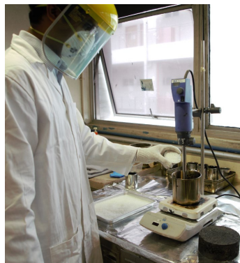
Performing wet mixing of waste plastics on bitumen at the laboratory.
