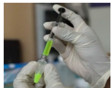
Preparation of fluorescence dye-encapsulated liposomes for functional studies of synthetic water channels (foldamers).
