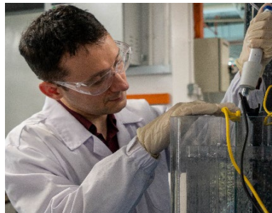
Purifying hard-to-treat industrial wastewater by electrochemical advanced oxidation process.
