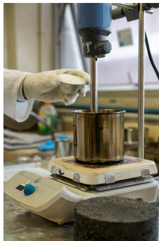
Asphalt sample with waste plastics wet-mixed into bitumen
