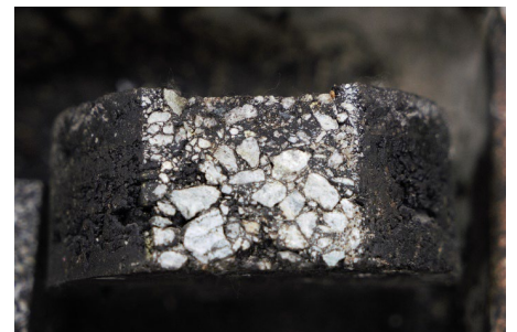
Asphalt sample with waste plastics wet-mixed into bitumen
