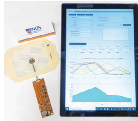
The VeCare platform comprises (clockwise from bottom left) a chip, wound sensor, bandage and app for real-time chronic wound monitoring. PHOTO: NATIONAL UNIVERSITY OF SINGAPORE
