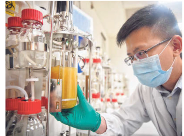
Above: NUS Medicine research fellow Garrett Wong fermenting engineered yeast in a bioreactor. After the fermentation, D-lysergic acid, a key ingredient for dementia drugs, can be extracted from the solution. ST PHOTO: JASON QUAH
