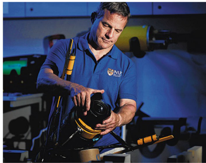
Dr Hoffmann-Kuhnt with the acoustic source position overlay device, or Aspod, an underwater recording device. The Aspod has a camera and three underwater microphones known as hydrophones. ST PHOTO: CHONG JUN LIANG
