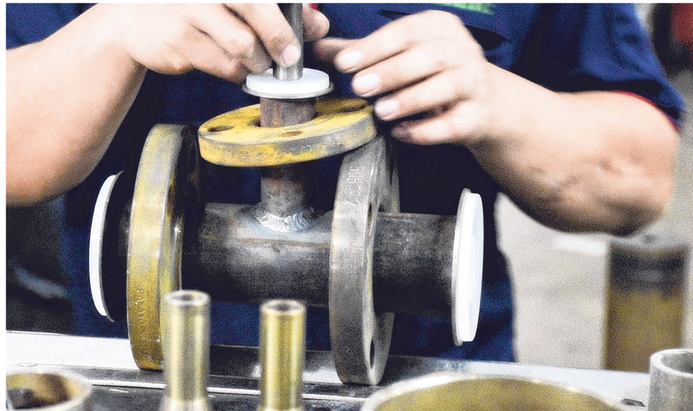
Almarc Engineering’s PTFE/PFA-lined pipes are carefully inspected before being fitted into customers’ manufacturing facilities. PHOTO: ALMARC ENGINEERING
