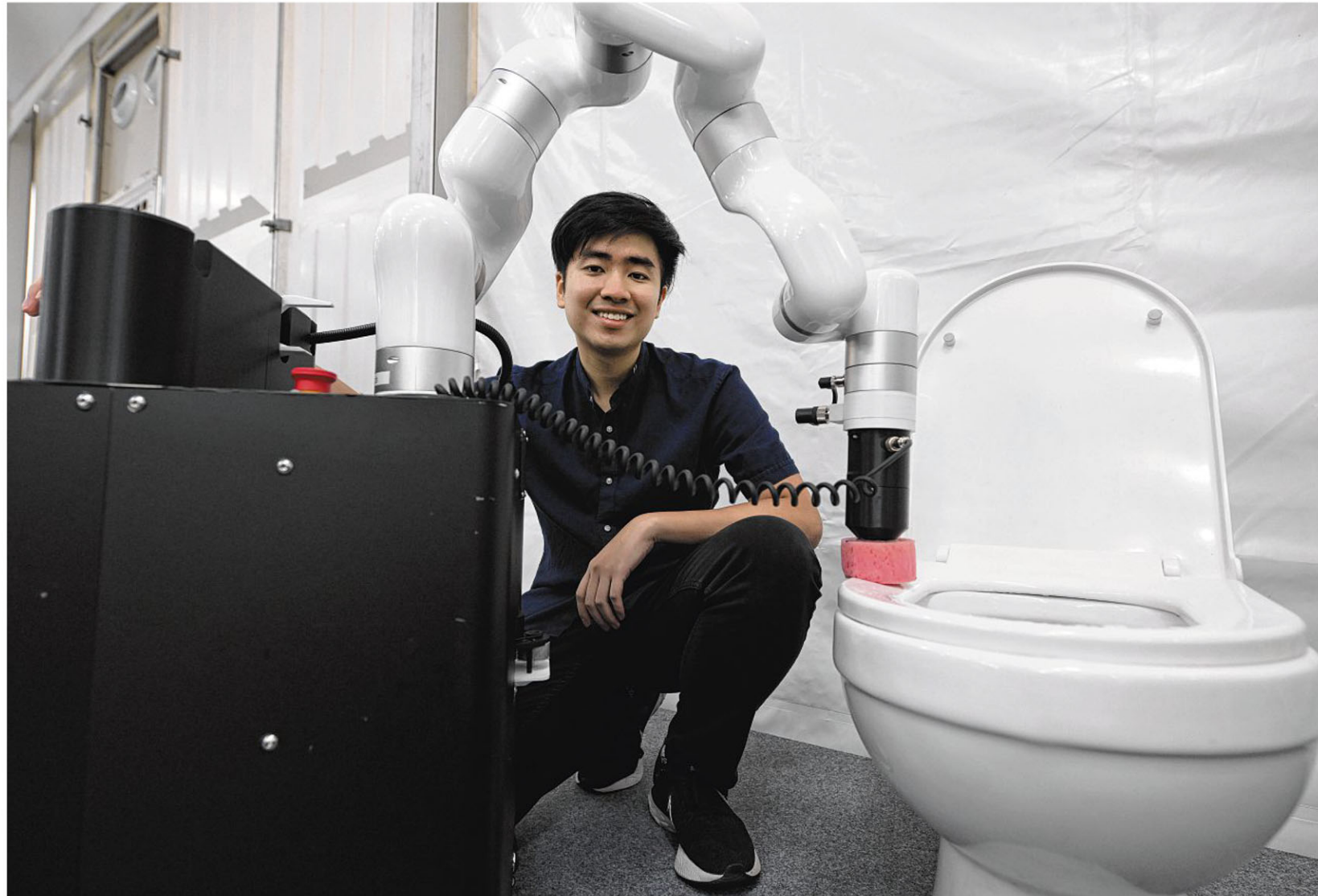
HiveBotics co-founder Tuan Dung Nguyen with his company's toilet-cleaning robot. It can move around a loo seeking out stains and areas to clean, guided by sensors that give it a 3D view of its surroundings. The robot's public testing phase will begin in the second quarter of 2024, marking the final stage of its development before its commercial launch in July, said Mr Nguyen. ST PHOTO: NG SOR LUAN
