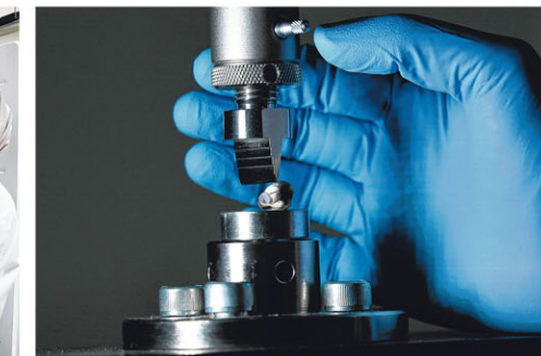
9 A test being conducted on the force required to remove dental fillings by shear stress on a tooth. This is done by simulating the biting action, which will cause the filling to fall off.
