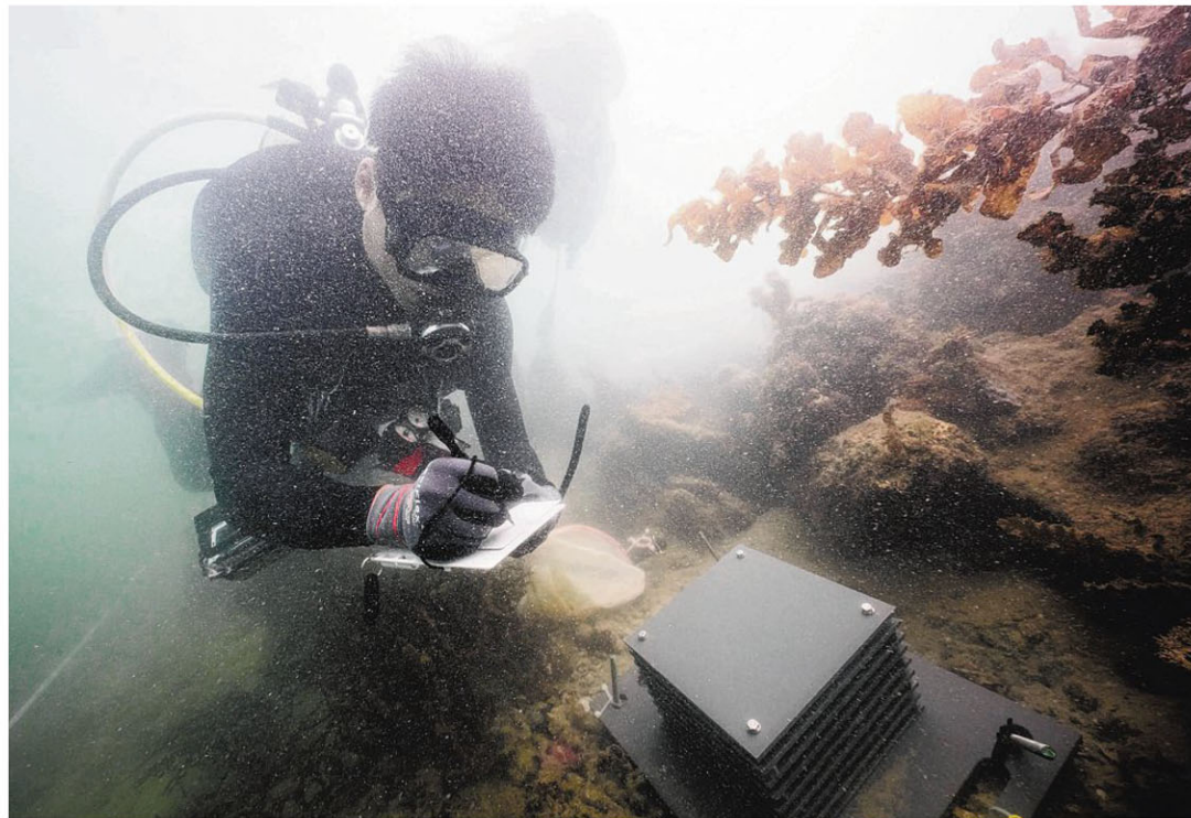
NUS marine biologist Huang Danwei noting down his observations after an Autonomous Reef Monitoring Structure (Arms) was installed on Oct 9. The 42 structures deployed in Singapore's southern waters will be left in place for one or two years, after which they will be taken back to the lab and examined. PHOTO: TOH XING JIE
