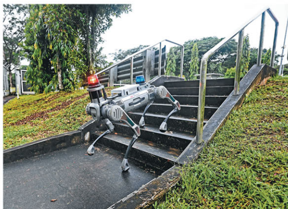
WATCH DOGS Mars, which patrols Seletar Bus Depot's perimeter fence, is armed with high-definition cameras, thermal imaging and other sensors to spot intruders and signs the fence has been tampered with. PHOTO: LIANHE ZAOBAO
