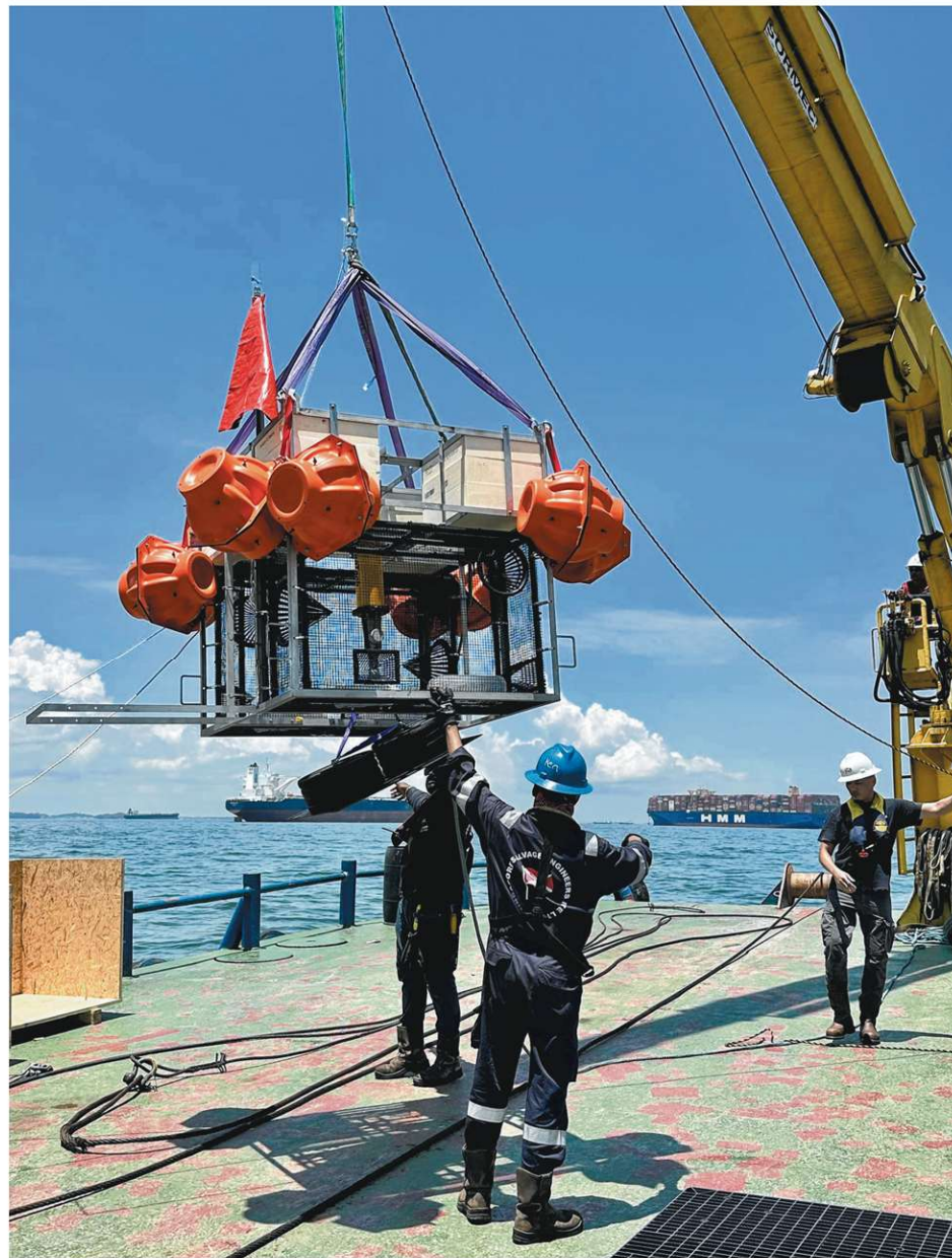
NUS researchers testing out a special system of "traps within a trap", which they plan to use to survey fish life during the expedition in October. The deepest depths that will be explored will be about 4,000m. PHOTOS: NUS
