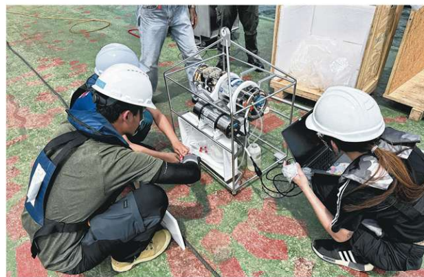
An environmental DNA (eDNA) sampler. Another innovation being piloted is the use of eDNA technology, which will allow scientists to detect traces of genetic material from coastal ecosystems, even in deep waters. It will also allow them to identify species and estimate the abundance of wildlife in the area.
