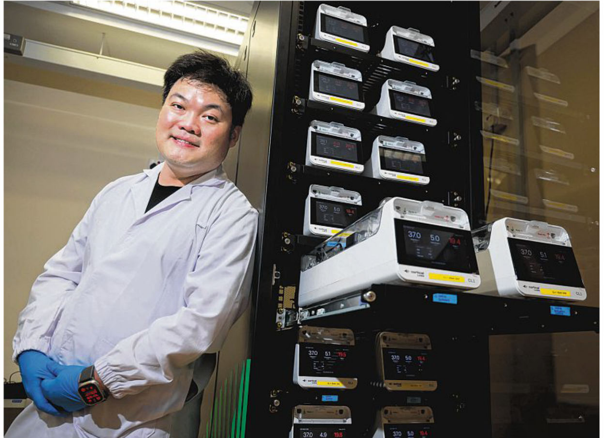
Chong Hon Weng, founder and chief executive officer of Cortical Labs, at the Cortical Cloud brain-cell powered data centre at NUS, on Aug 7. Beside him is a rack of 20 units of biological computers. Each unit houses at least 200,000 lab-grown neurons sitting on an electrode-fitted silicon chip. ST PHOTOS: JASON QUAH
