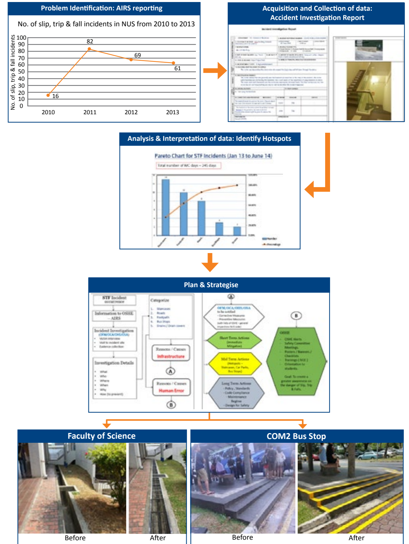
Figure 3.1.4 Application of knowledge management in reducing slip, trip and fall incidents: identification of problem, data acquisition and analysis, working with partners to resolve the issues, and strategising action plans to reduce STF incidents
